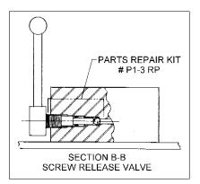
If the valve fails to operate properly after cleaning it may be necessary to re-seat the valve balls. Remove the springs and tap each ball lightly in its respective seat using the 1/4" ball seating tool (CP13-42) for the small ball and the 3/8" ball seating tool (CP13-43) for the large ball. Remove balls to make sure they are not stuck to the seats. Reassemble pump valve as before..
