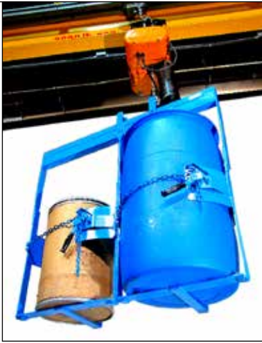
Custom Model # 86S-2D for 2 drums Capacity: 2000 Lb. (907 kg) total, 1000 Lb. (454 kg) per drum
