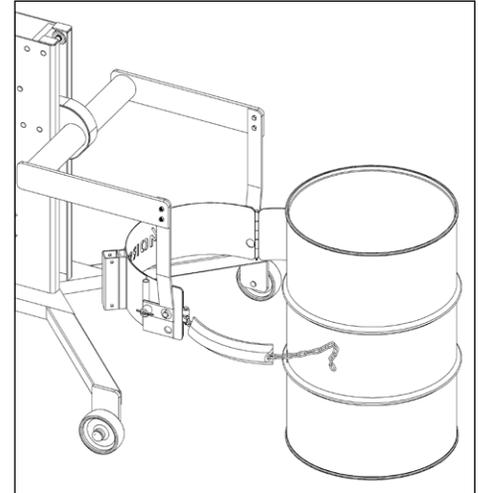
4. Either one of the two spring loaded plunger tilt locks may be locked to hold drum upright. Unlocking both will permit drum to be tilted. Drum pouring angle may be varied or drum can be locked in horizontal position by inserting one tilt lock. It is not necessary to lock both tilt locks. Before unlocking tilt lock it is recommended that you steady drum and prepare to resist its tendency to tilt toward its heavy end.
