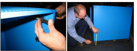
Step 9: Adjust the three casters so bottom of cage is approximately 4" off the floor (shown right). Do not lock in place just yet. Close enclosure and verify that the key aligns properly with the switch. If key is not aligned properly adjust casters accordingly. Key may also be adjusted by loosening its screws and moving (shown left). Once key is aligned properly, lock casters in place by tightening jam nut upward.
