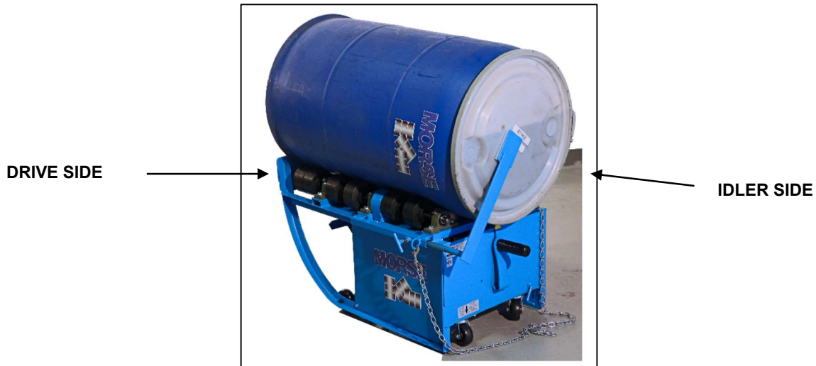
Morse Portable Drum Roller Shown with Kit POLY-201FI Installed
