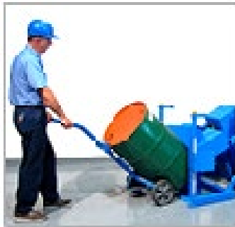
Figure 5.1 Load drum with drum truck
