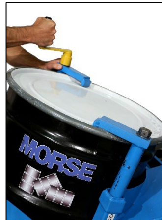
Figure 5.5 Turn the top clamps until they tighten against top of drum. Then remove hand crank BEFORE rotating drum.
