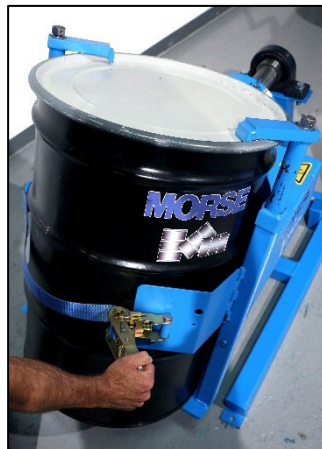
Figure 5.4 Drape the web strap across the face of the drum, and thread through slot in ratchet. Operate ratchet to tighten strap around drum.
