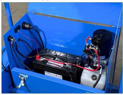
Inspect the hydraulic system for oil drips, hose damage, or other signs of wear. Inspect the level and condition of the hydraulic fluid. Replace any parts that show signs of wear.
