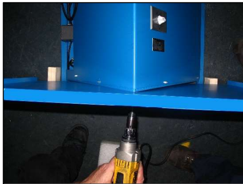
Step 8: Screw 5 self drilling screws through back panel and into the angle frame.
