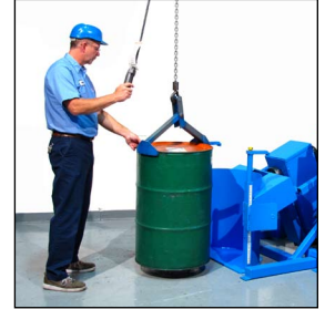
Load drum with hoist attachment
