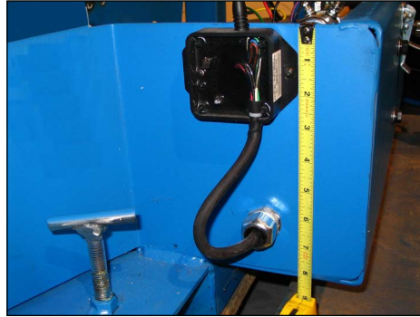
6. Layout receiver and drill (1) 7/8" diameter hole and (2) 1/4" diameter holes per picture.
