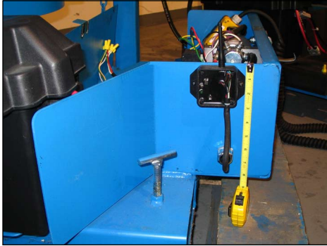
6. Layout receiver and drill (1) 7/8" diameter hole and (2) 1/4" diameter holes per picture.
