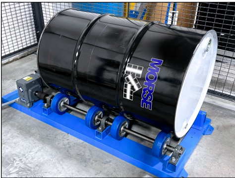
Position drum with ribs between roller wheels.
