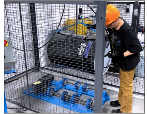
Lower horizontal drum onto drum roller.
