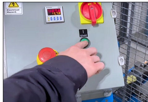
Push START button to begin drum rolling.
