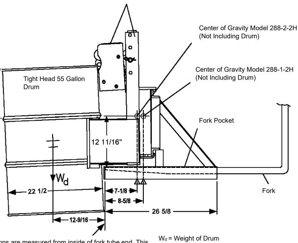
Dimensions are measured from inside of fork tube end. This will give a fixed point to which lost load data can be determined. Forks must be touching this fork tube end.
