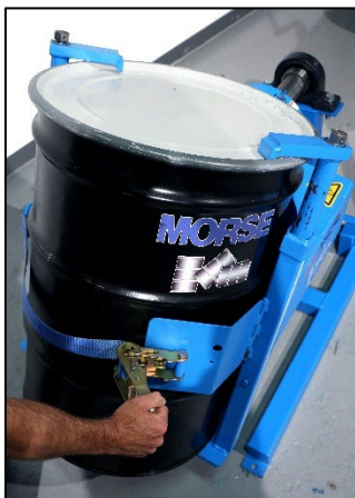
Figure 4.1 load drum with hoist using appropriate drum lifting equipment, such as model 92 Drum Lifter
