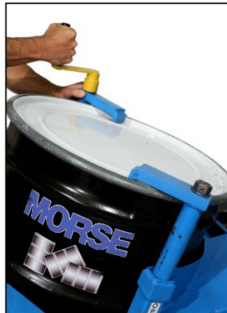
Figure 4.4 Turn top clamps until they tighten against top of drum. Remove hand crank BEFORE rotating drum.
