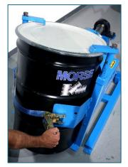
3. Drape the web strap across the face of the drum, and thread through slot in ratchet. Operate ratchet to tighten strap around drum.
