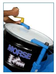
4. Turn the top clamps until they tighten against top of drum. Then remove hand crank BEFORE rotating drum.
