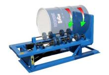
5. The drum rotation speed can be varied with the metering valve. Turn the valve clockwise to increase drum 16 RPM. Turn valve counter-clockwise to decrease drum RPM.
