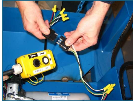
12. For pendant operation, plug male plug from pendant into female plug of pump.
