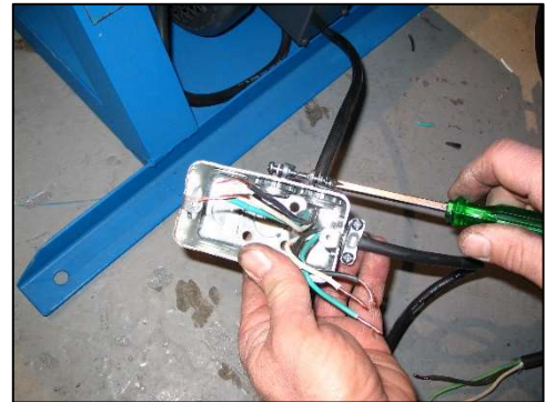
Step 7: Install safety switch wire through the middle side hole. Tighten screws.
