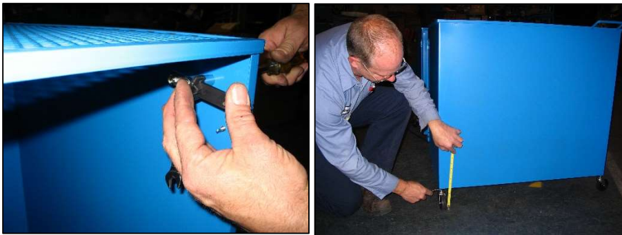
Step 9: Adjust the three casters so bottom of cage is approximately 4" off the floor (shown right). Do not lock in place just yet. Close enclosure and verify that the key aligns properly with the switch. If key is not aligned properly adjust casters accordingly. Key may also be adjusted by loosening its screws and moving (shown left). Once key is aligned properly, lock casters in place by tightening jam nut upward.
