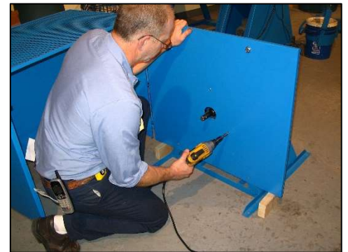
Step 9: Adjust the three casters so bottom of cage is approximately 4" off the floor (shown right). Do not lock in place just yet. Close enclosure and verify that the key aligns properly with the switch. If key is not aligned properly adjust casters accordingly. Key may also be adjusted by loosening its screws and moving (shown left). Once key is aligned properly, lock casters in place by tightening jam nut upward.
