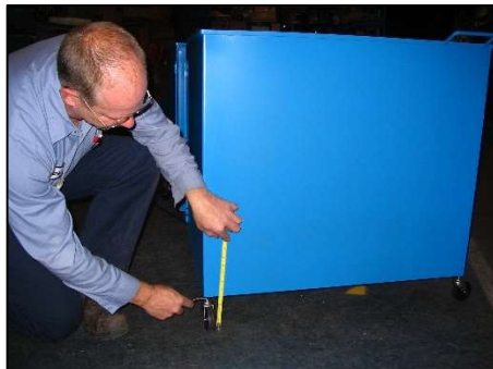
Step 9: Adjust the three casters so bottom of cage is approximately 4" off the floor (shown right). Do not lock in place just yet. Close enclosure and verify that the key aligns properly with the switch. If key is not aligned properly adjust casters accordingly. Key may also be adjusted by loosening its screws and moving (shown left). Once key is aligned properly, lock casters in place by tightening jam nut upward.
