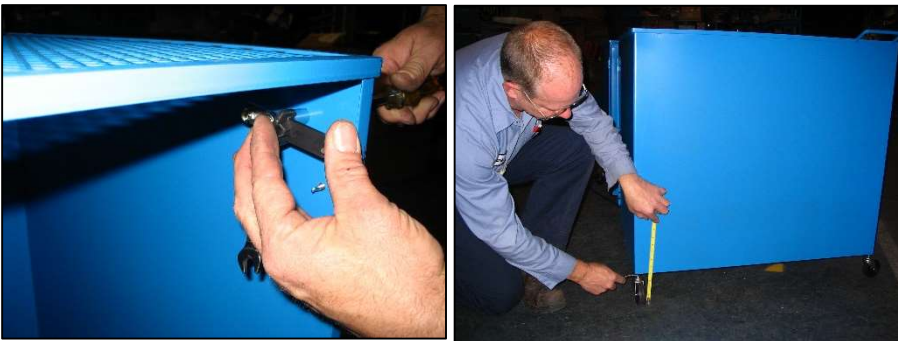
Step 9: Adjust the three casters so bottom of cage is approximately 4" (102mm) off the floor. Do not lock in place yet. Close enclosure and verify that the key aligns properly with the switch. If key is not aligned properly adjust casters accordingly. Key may also be adjusted by loosening its screws and moving. Once key is aligned properly, lock casters in place by tightening jam nut upward.
