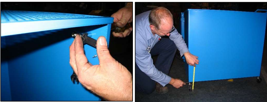
Step 9: Adjust the three casters so bottom of cage is approximately 4" (101.6mm) off the floor. Do not lock in place yet. Close enclosure and verify that the key aligns properly with the switch. If key is not aligned properly adjust casters accordingly. Key may also be adjusted by loosening its screws and moving. Once key is aligned properly, lock casters in place by tightening jam nut upward.
