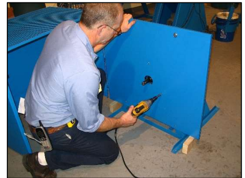
Step 9: Adjust the three casters so bottom of cage is approximately 4" (101.6mm) off the floor. Do not lock in place yet. Close enclosure and verify that the key aligns properly with the switch. If key is not aligned properly adjust casters accordingly. Key may also be adjusted by loosening its screws and moving. Once key is aligned properly, lock casters in place by tightening jam nut upward.
