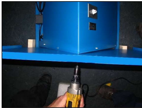
Step 8: Screw 5 self drilling screws through back panel and into the angle frame.
