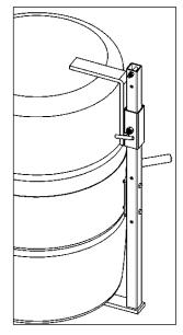
Figure 2.1 Plastic drum being lifted with part number 4556M-P Bracket Assembly installed.
