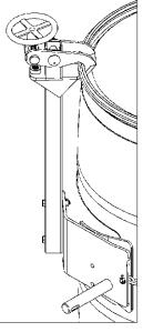
Figure 2.2 Plastic drum being lifted with part number 4560M-P Top Rim Clamp Assembly installed.
