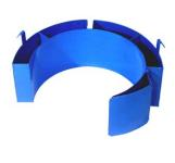
Diameter Adaptors for drums from 18.5" to 22" (47 to 55.9 cm) in diameter do not have hold-down brackets. They fit between the ribs of a steel drum. For plastic or fiber drum, use Diameter Adaptor in combination with the Bracket Assembly to prevent the drum from slipping lengthways through the drum holder.
