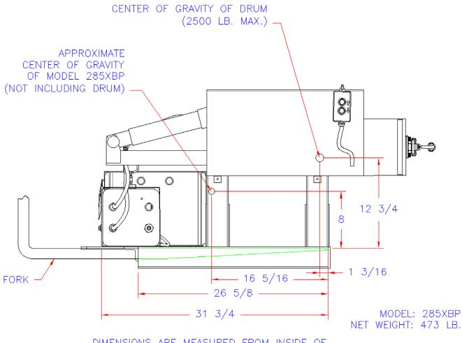
DIMENSIONS ARE MEASURED FROM INSIDE OF FORK TUBE END. THIS WILL GIVE A FIXED POINT TO WHICH LOST LOAD DATA CAN BE DETERMINED. (FORKS MUST BE TOUCHING THE FORK TUBE END.)
