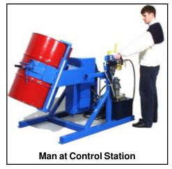
Each function is controlled separately by levers mounted on the control station (see figure above):
