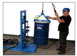
3. Lower the "TILT" lever to tilt the drum from upright into horizontal position.
