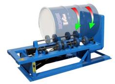
5. The drum rotation speed can be varied with the metering valve (item 13 on page 8). Turn the valve clockwise to increase speed up to 20 RPM, counterclockwise to decrease speed down to 5 RPM.
