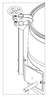
Figure 1 Plastic drum being lifted with part number 4560M-P Rim Clamp Assembly Kit installed.
