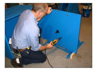
Step 9: Adjust the three casters so bottom of cage is approximately 4" off the floor. Lock casters in place by tightening jam nut upward.
