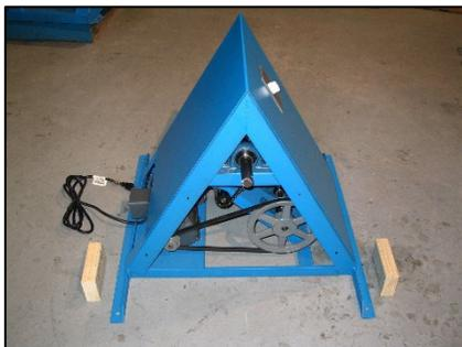
Step 5: Place a 2 x 4 spacer on each side of the frame, these will be used to hold the back panel of enclosure 3-1/2" off the floor.
