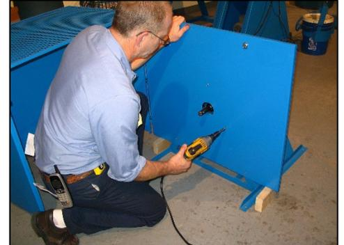
Step 9: Adjust the three casters so bottom of cage is approximately 4" off the floor (shown right). Do not lock in place just yet. Close enclosure and verify that the key aligns properly with the switch. If key is not aligned properly adjust casters accordingly. Key may also be adjusted by loosening its screws and moving (shown left). Once key is aligned properly, lock casters in place by tightening jam nut upward.
