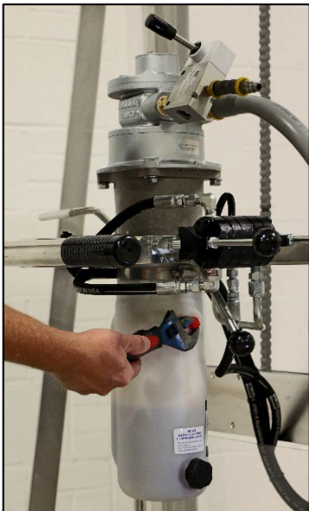
Remove RED shipping plug from the hydraulic reservoir
