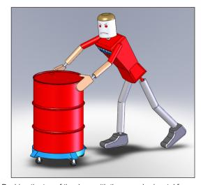
Pushing the top of the drum with the same horizontal force will result in a 73% load shift to the front wheels of the dolly. The dolly can become difficult to control and potentially hazardous - even tip over, especially if the dolly wheels hit an obstruction, a hole in the floor, or you descend a slope.
