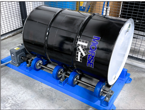
Position drum with ribs between roller wheels.
