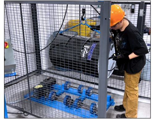
Lower horizontal drum onto drum roller.
