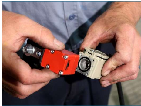
If necessary, reverse orientation of switch. . .
