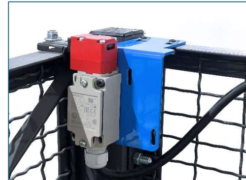
Close enclosure and verify that the key aligns properly with the switch. If key is not aligned properly, adjust accordingly. Key may be adjusted by loosening its screws and moving, then re-tightening screws. Use zip ties to retain cable from switch to control station.
