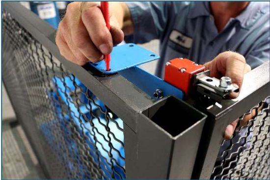
Mark where to drill holes in top of side panel for switch mounting plate.
