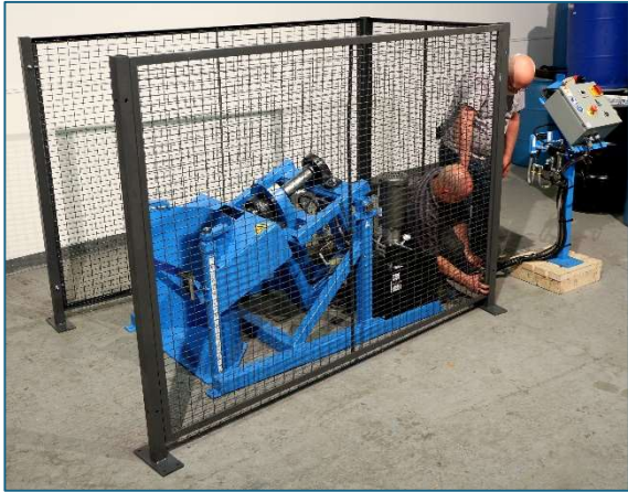
Attach enclosure end panel to posts with provided hardware.
