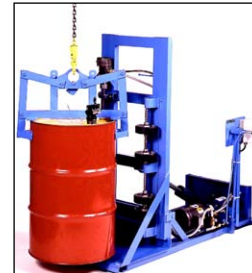
Load drum with hoist attachment
