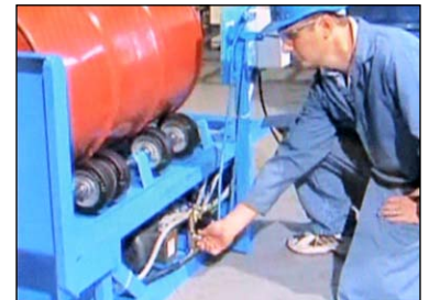
Vary the rotation speed with the flow control valve
