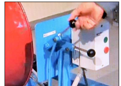
Raise the "ROLL" lever to begin rotation
