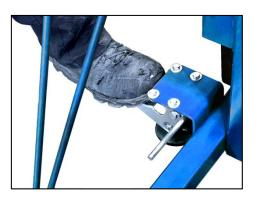
Adjust height of rim catch to pail top and tighten in place to prevent pail from 3. slipping while pouring. If the pail has pivoting wire handle, swing it to lay on front side to clear back band of holder.
