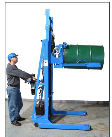
4. Release clamp. Then raise horizontal drum to proper height to place on rack up to 8.5' (2.59 m) high.
