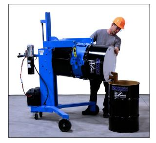
This innovative design combines the V-shaped base to serve the corner of a pallet, with a drum holder to rotate and dispense a drum.
