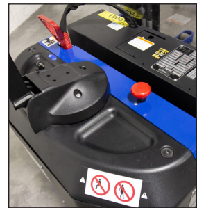
Quick-disconnect battery plug and dead-man brake safety features.
