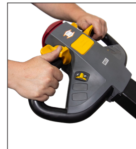
Familiar Controls for propulsion and steering. Raise and Lower Buttons also incorporated in handle.
