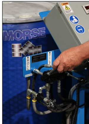
8. Use the ROLL handle to begin drum rotation
