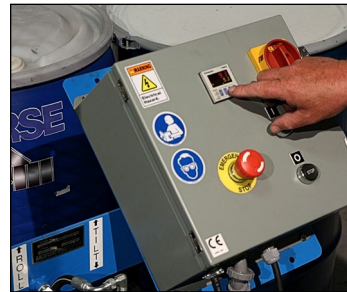
6. Set timer to rotate drum for desired time, from just a few seconds... up to 16 hours
