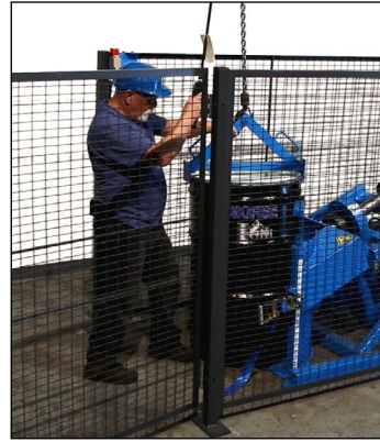
1. Load your upright drum at floor level with a drum truck or below-hook drum lifter
