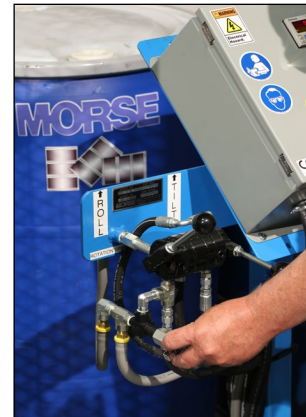
9. Adjust drum rotation from 4 to 16 RPM
