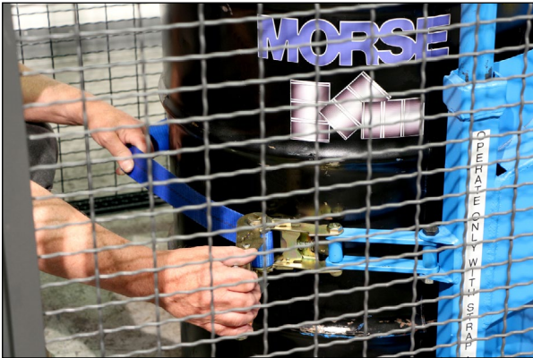
2. Secure drum in holder with ratchet strap. . .
