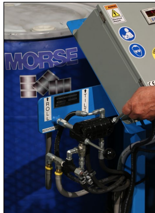
7. Use TILT handle to raise the drum into rotating position
