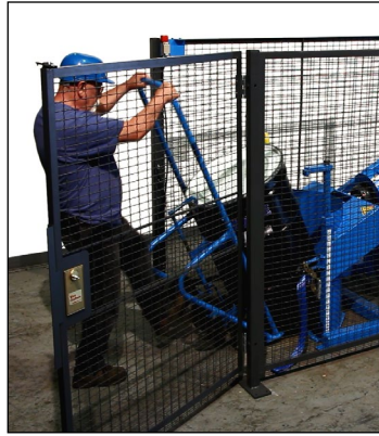
1. Load your upright drum at floor level with a drum truck or below-hook drum lifter
