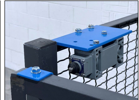
Morse Switch Assembly (Kit 3597KIT-P) installed at enclosure gate opening
