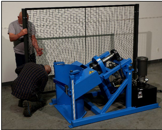
Attach enclosure side panels to posts with provided hardware.
