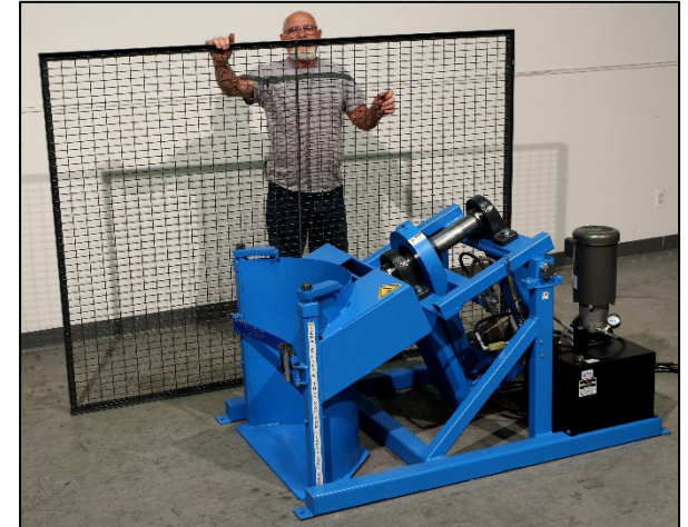
Position the drum rotator at the desired location, ensuring there is ample room for enclosure, and for loading a drum onto the drum rotator.
