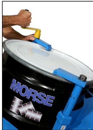
Figure 4.4 Turn top clamps until they tighten against top of drum. Remove hand crank BEFORE rotating drum.
