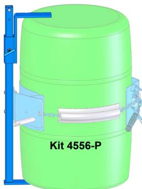
Install **Bracket Assembly Kit 4556-P** to prevent drum from slipping length-ways. Required to safely handle a RIMLESS 55-gallon (210 liter) plastic drum. Also recommended to more securely hold fiber drum. Adjusts for 31" to 39" (78.7 to 99 cm) tall drum.
