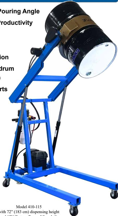
Model 410-115 with 72" (183 cm) dispensing height and 12V Battery Power lift and tilt
