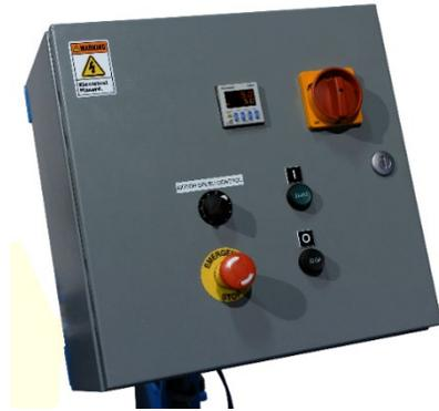
NON-explosion proof AC Control Packages (sold separately) include control box with timer, start and stop buttons, emergency stop button and lockable main disconnect. 309-1 control packages offer fixed speed of 14 rpm. 309-3 control packages (shown) offer variable speed control from 2 to 20 rpm.
