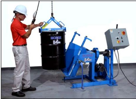
Load drum with hoist using appropriate drum lifting equipment, such as model [92 Below-Hook Drum Lifter](#).
