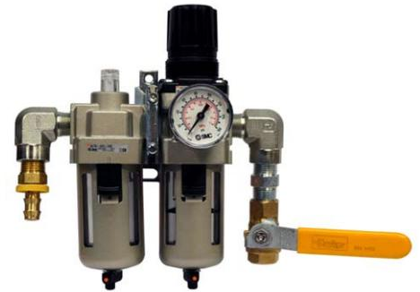
Morse Air Control Package (included with model 309-A) includes Filter, Regulator, Lubricator (FRL) and on / off valve. Drum Tumbler rotates drum at 14 RPM and allows you to vary RPM with air flow and pressure.
