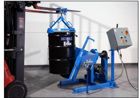
Load drum with forklift, using appropriate drum lifting equipment, such as Morse [model 284 Fork Hook](#) and model [92 Below-Hook Drum Lifter](#).
