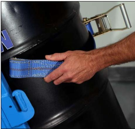
Place loop of web strap onto clevis
