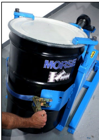
Figure 4.3 Drape web strap across face of drum. Thread strap through slot in ratchet. Operate ratchet to tighten strap around drum.
