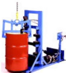
Loading drum onto Model 456 with Morse Model 90 Verti-Karrier
