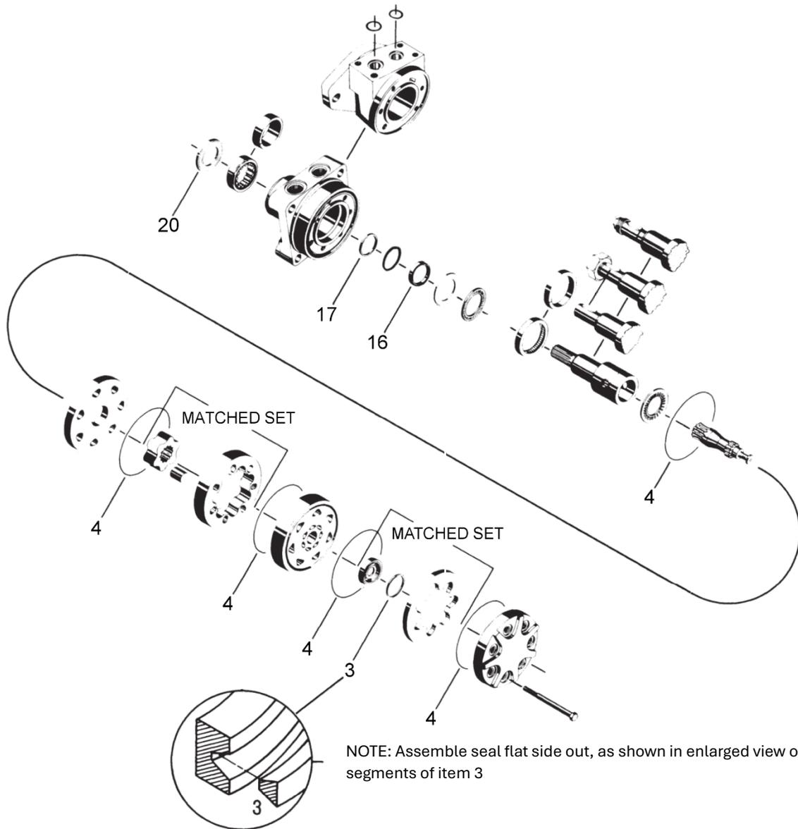
NOTE: Assemble seal flat side out, as shown in enlarged view of sectioned segments of item 3
