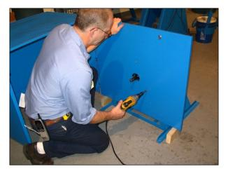
Step 9: Adjust the three casters so bottom of cage is approximately 4" off the floor. Lock casters in place by tightening jam nut upward.
