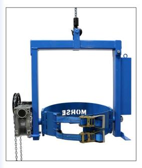
Manual drum tilt is controlled with a 12' (366 cm) pull chain loop hanging 6' (183 cm) below the chain wheel. There is enough resistance in the enclosed gear box to automatically stop and hold the drum tilt angle. Hand wheel tilt control option is also available.
