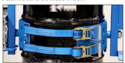
while letting out other side to turn drum. Chain loop provides control of drum tilt 360° in either direction, even while drum is hoisted above reach.
