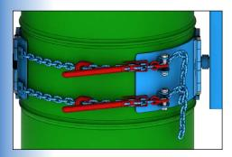
Option # 6214i-P Factory installed Chains and Load Binders Kit # 6214-P
